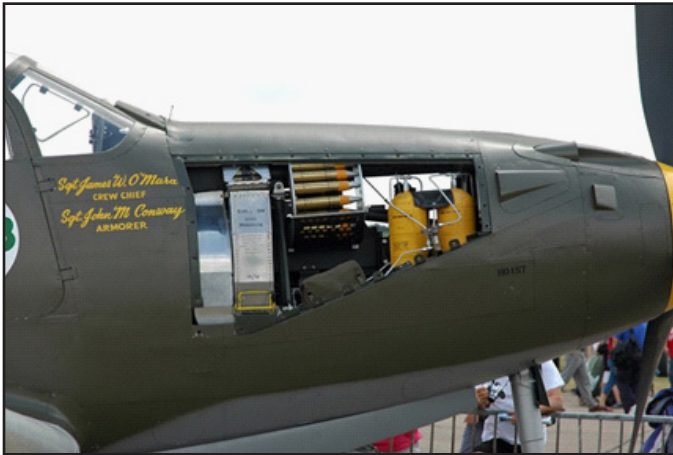
The 37mm Oldsmobile T-9 in a restored P-39
